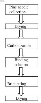
The pine needles briquettes bonded with less amount of clay are more efficient and have high calorific value, generate less smoke and ignition takes place properly.
